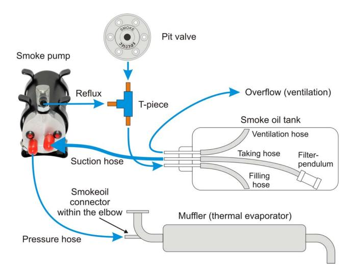
The suction hose is often an unattended area. For a flow rate of 740ml/min. or more, the suction hose must not be arbitrarily long. Retrieve the maximum suction hose length and minimum diameter from table 1 for your desired flow rate. Observe that the suction hose starts with a pendulum in the tank. Values in the table refer to the total length which includes the pendulum length.
