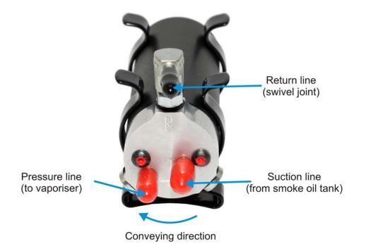
Flow direction is marked by an arrow. The "R" marked connector (swing fixture) is to be routed back to the tank. Back flow is approx. 35ml/min. In order not to install a separate connector to the tank, a delivered T-piece can be looped into the tanking hose. Here, the back flow is to be connected.
