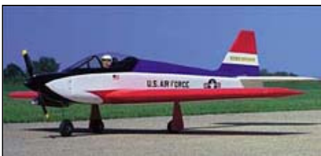
DKM-235AC Kougar Black Lettering Decal. "USAF" letters are 3" high, "U.S. Airforce" is 1" high x 9-1/2" long, the buzz numbers are 13/16" high.
