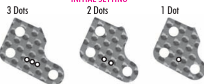
Steering angle of the OUTSIDE wheel.
