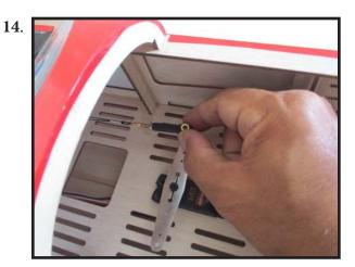
Crimp the brass swage tube with a crimping tool or pliers.
