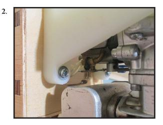
Reinstall the servo horn by sliding the connector over the pushrod wire. Center the throttle stick and trim and install the servo horn perpendicular to the servo center line.
