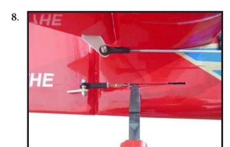
Cut off excess cable as shown.
