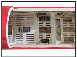
Feed one rudder cable through the pre installed cable exit tube in the rear of the fuse toward the front of the fuse. Repeat for other side.
