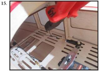
Cut off excess cable as shown.
