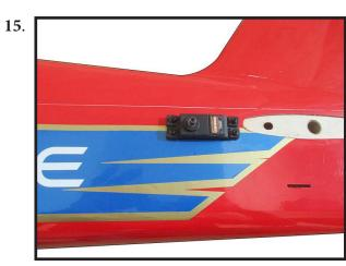
**Maximum Servo spec. Torque :** 102 oz-in (7.3 kg-cm) @ 6.0V;
