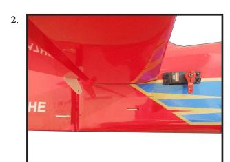
Thread the rudder cable through a brass swage tube, then the threaded co pler, and back through the brass swage tube on both sides. Pull light tension on the cable through the coupler on both sides as shown.
