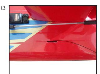
Thread cable through brass swage tube.
