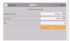
When the "RX Connected" page pops up, press the [REGISTER] to complete the Registration procedure and then power the receiver off.
