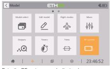
Enter the RF system menu by the touch-screen or use the navigation encoder key.
