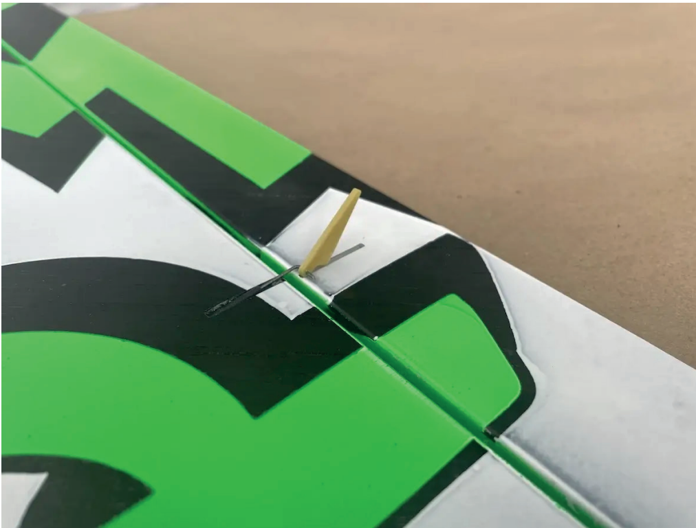
Install control horns onto the L-bands and glue the last in place.
