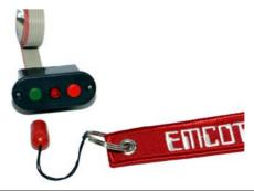
The central, ultra-bright light-emitting diode (LED) in the switch transmitter always illuminates when the **DPSI** is switched on. In case of an error (e.g. low voltage) or during programming the LED indicates the states through different blink codes.
