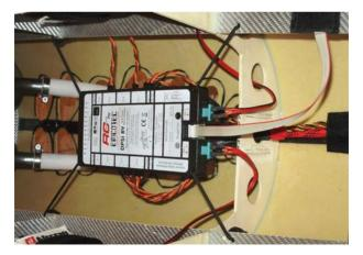
Generally, you must always ensure that the fastening is as vibrationfree as possible and has sufficient air circulation. Reduction of vibration is particularly important for the receiver, since it reacts far more sensitively to mechanical vibrations than the **DPSI**.
