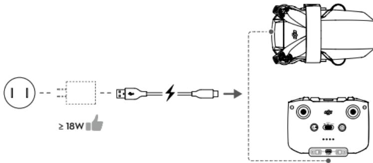
EN Charge to activate the Intelligent Flight Battery before using for the first time.
