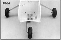
85. Install a 3/4" dia. tailwheel on the tailwheel wire using two 1/16" wheel collars (not included SIGSH584). A cleaner, but more difficult installation would be to solder small flat washers to the wire on both sides of the tailwheel. Solder the inner washer first, then slide the tailwheel in place followed by a temporary spacer made from thin cardboard. Solder the remaining waher, then remove the spacer when cool. Whether you use wheel collars or washers, trim off any excess tailwheel wire.
