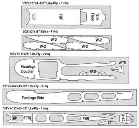
Leave all die-cut parts in the sheets until needed in construction. Then remove the pieces from the sheets carefully. If difficulty is encountered, do not force the part from the sheet - use a modeling knife to cut it free.
