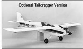
weight (no nose gear), resulting in increased performance. The tail dragger version handles very well on the ground - if you've always wanted to try a taildragger, this would definitely be a good one to start with.
