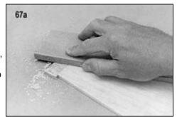
68. With the elevators still taped to the stabilizer, use a sanding block to round off the stab leading edges, stab tips, and elevator tips. Notice that the short length at the front of the stab should be left flat to fit against the back of F-6.
