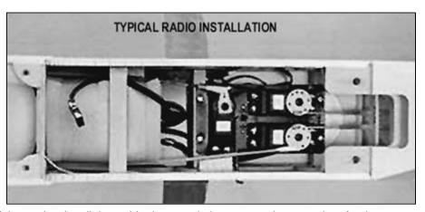
loads.) Thread the R/C link onto the end of the pushrod until the rudder is neutral, then repeat the procedure for the elevator .
