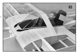
a. Remove the canopy assembly from the model and trim away the canopy base flush with the edge of the flange on the canopy. Sand the edges smooth leaving about a 3/32" flange on the sides of the canopy.
