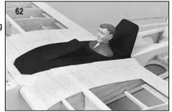
a. When you're satisfied with the finish of your canopy interior, tape the assembly back in position along the outer edges of the canopy base.
