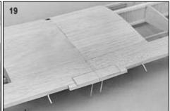
19. Glue the 1/16"x3/4"x1-1/2" plywood wing hold-down plates to the top of the wing, even with the back of the torque rod blocks.
