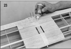
Remove the tape from the servo cutout area after the glue is dry.
