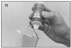
NOTE: Epoxy may be used in this step, but CA is faster and penetrates the entire tailwheel area, making it rock hard.
