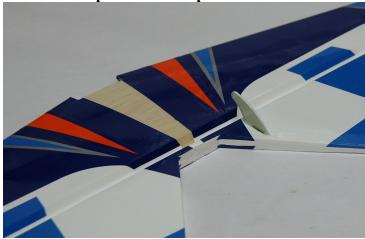
13. Center the hinges in their slots and secure with a couple drops of fresh thin CA on each side of the hinge. Strive for the smallest hinge gap possible.
