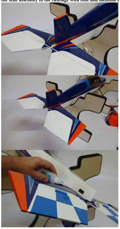
15. Scuff the rudder horn with sandpaper and glue into the pre-cut slot on the lower portion of the rudder with medium CA. Slide the rudder onto the hinges and secure to the fuselage with thin CA.
