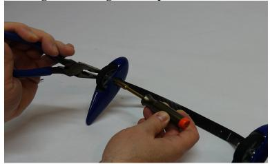
5. Mount the landing gear assembly to the fuselage using the provided 3mm socket head cap bolts and washers. Make sure to apply a drop of blue thread lock compound to the bolts.
