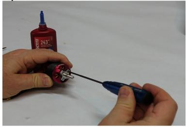
9. Attach the motor to the front of the motor box with the supplied 3mm socket head cap bolts.
