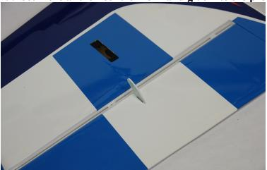
20. Center the hinges in their slots and secure the aileron to the wing with thin CA. Repeat this process for the other wing.
