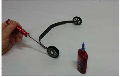
4. Slide the wheel pant into position. Tighten the nut on the axle so that the wheel pant is pinched between the axle and the landing gear leg. The recessed area of the wheel pant will align with the gear and prevent it from rotating. Repeat for the other wheel pant.
