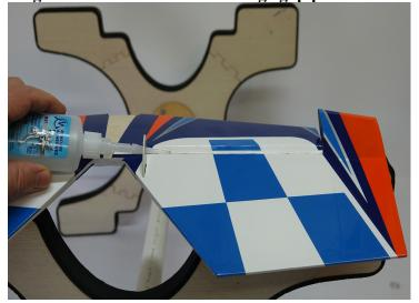
14. Insert the stab into the rear of the fuselage and push as far forward as possible. Slide the main wing tube into its sleeve to check alignment with the stab. Measure side to side as well. When satisfied secure the stab assembly to the fuselage with thin and medium CA.
