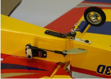
19. Scuff the aileron control horn and glue into the pre-cut slot with medium CA.
