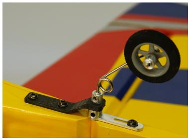
17. Attach an 18" Extreme Flight 28AWG servo extension to the elevator servo lead and secure with heat shrink tubing or an Extreme Flight servo extension lock. Install the elevator servo into its slot and assemble the linkage as shown. There is a G10 servo arm included in the hardware package, used to achieve 3D throws in excess of 50 degrees. Attach this arm to the stock servo arm with a 2mm screw and nut as shown. Use your power drill to help thread the ball links onto the pushrod.
