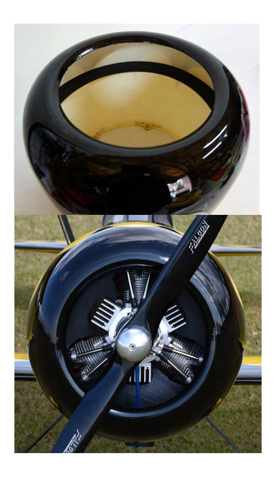
22. Make an opening in the bottom of the cowl to allow incoming air to exit. Below is a picture of the cutouts I made on the bottom for the gas twin engine version for the exhaust stacks and air exit. I made a similar opening on the radial version.
