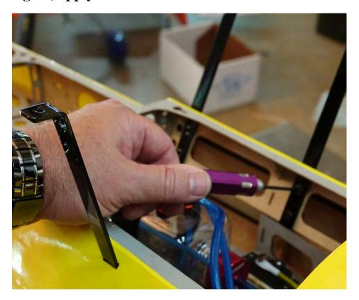
17. Mount a 24 ounce Flowmaster gas tank on the tank tray and run your fuel line (carb feed, fill tube, overflow). Install an EF Fuel Dot for easy fueling/defueling.
