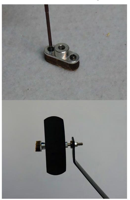
10. Slide the wheel pant into position and secure with 2 3mm socket head cap bolts, inserted through a washer, the carbon gear and into the blind nuts in the wheel pant. Again, use Blue Loctite on these bolts and tighten securely.
