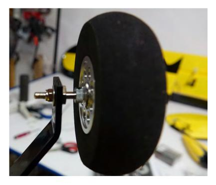
9. Attach the aluminum wheel pant bracket to the wood spacer with the included black wood screws. Retain the wheel with the bracket assembly as shown. Be sure to use Blue Loctite on the grub screw.
