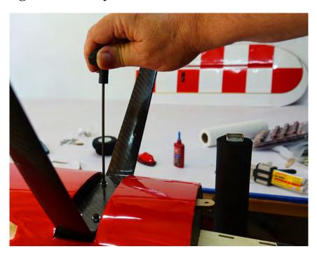
7. Slide the landing gear fairings into place and mark the landing gear with a felt tip marker to show where they fit. Remove the cuffs and lightly scuff the carbon gear for maximum glue adhesion. Use epoxy or "Goop" silicon adhesive to permanently attach the fairings to the gear. I suggest using blue painters tape to keep the fairings securely in place while the adhesive sets.
