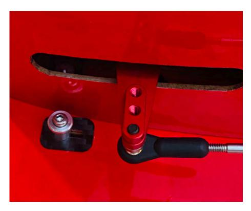
25. Slide the wing tubes into the fuselage and center wing section. Open the latches in the fuselage and bottom of the upper center section. There is a rod spring in the lower wing latch that must be depressed for the latch to open. This can be done with the tip of your finger or a small flat blade screw driver. Slide the wing into position, connect your servo leads and push the latch into the closed position.
