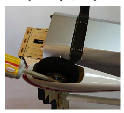
12. Drill a hole in the bottom of the rudder to accept the ball link included in the tailwheel assembly package. Scuff the shank of the ball link with sandpaper and glue it into the hole with epoxy or medium CA. Slide the tailwheel tiller arm into the hole in the ball link and bolt the assembly to the bottom of the fuselage.
