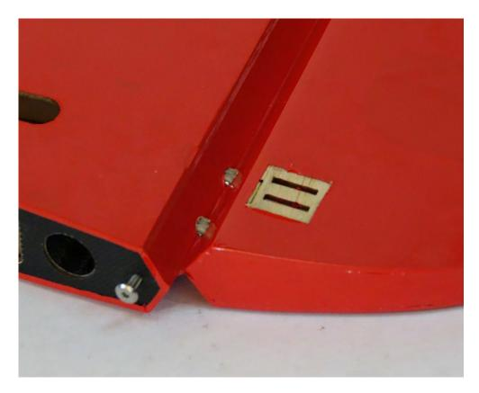
3. Test fit the control horns and baseplate into the surface and make sure everything fits properly. Use a high quality epoxy to glue the horns into the surfaces. I've started using the Loctite Hysol products and glue gun which makes this process so much faster with less clean up required and less waste. I like the slow set EA 9462 for this particular procedure. It allows plenty of time for gluing all of the control horns into place in one sitting.
