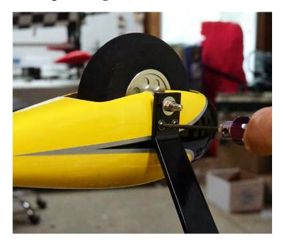
11. Pull the outer side of the pant away from the wood bracket and apply a bead of epoxy to the bracket. This will secure the pant mounting bracket to the fiberglass wheel pant, making a much stronger assembly.
