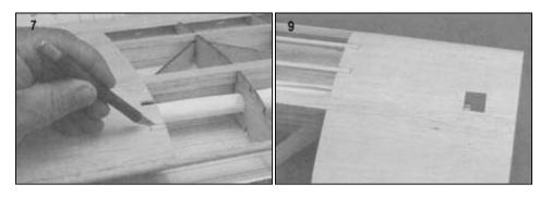
BE ABSOLUTELY POSITIVE THE SHEAR WEBS ARE BONDED TO BOTH THE TOP AND BOTTOM SPARS.
