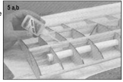
Trim one edge of a 3/32"x2"x36" balsa trailing edge sheet straight. For this step it is recommended that you apply SIG-Bond to the top of the trailing edge, and the ribs. Pin the trailing edge sheet and the trailing edge to the board to keep them straight until the glue cures.
