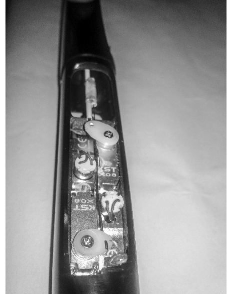
An example of servo mounting on the tray
