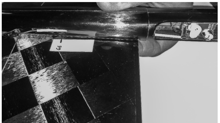
Start the linkage build from ailerons and finish it at the servo horn.
