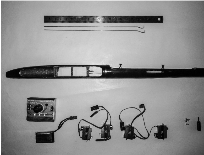
Check the neutral position of servos with a servo tester
