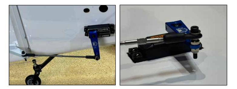
We recommend a 2" length servo arm for the rudder, as we do for the elevators. In our testing, on most brands of servos and radio systems, we are able to use the 1.75" location on the arm and achieve full throw with maximum torque and resolution. Please check this during your servo throw setup. On some setups, we can even use a 1.5" location on the rudder, but this is dependent on the individual pilot's preference for rudder throw, so this is an option to examine during flight testing.
