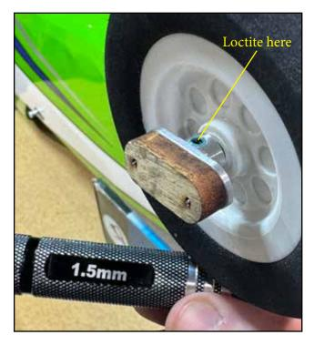
Install the wheel pant over the wheel and axle, apply loctite and start the M3 screws which retain the pant to the gear, but do not tighten.
