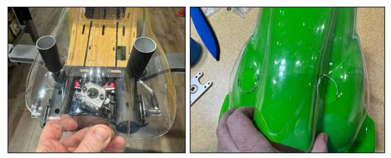
If you are using stock, in-cowl mufflers, you have the option to open the port in the bottom front of the fuselage, or not. The only reason not to open it is if you will use a smoke system. Leaving it closed can help to keep smoke oil residue out of the fuselage, however in this case you may need to cut some cooling vents in the bottom of the cowl to exhaust muffler heat. If you are not using smoke, definitely open this port and open the cooling holes on the bottom of the fuselage.
