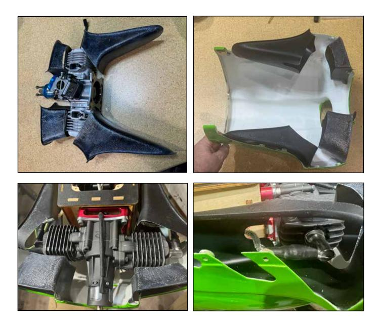
For outrunner electric setups, it is easy to convert the gasoline ducting to work. Cap the rear of the inlet ducts with balsa or foam and cut the inner wall of the duct to allow the air to escape toward the motor.
