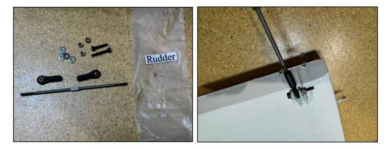
The rudder servo fits into the side of the fuselage in the pre-fabricated mounting locations as shown. On ALL mounting locations on the Peregreine, the opening should be tight to the servo body, you may need to open the location by a tiny amount to fit your particular servo, as the sizes of servo bodies are not precisely standardized. See the proper attachment of the pushrod on the servo arm side. It includes a cone-shaped spacer and locking nut, attach all pushrods to servo arms in this way.
