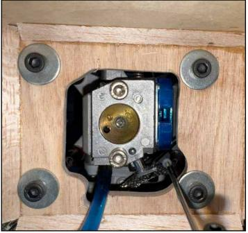
Mount the throttle servo as shown.
