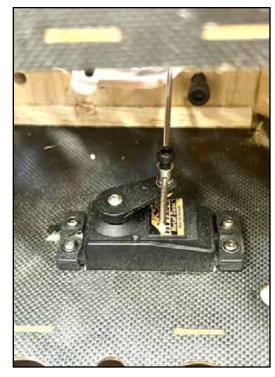
There are many options for choke actuation. You can run the linkage to the rear, you can install a choke servo; here we show a very simple forward choke rod installation. A forward choke rod may need a middle support, one convenient method is to make an "x" from zip ties around the engine standoffs, see photo. Install your fuel filler dot as shown.
