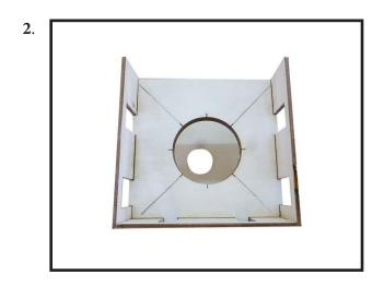
Attach the motor mount to the front of the electric motor box using four 5mm blind nut, four M5x30mm hex head bolts to secure the motor. Please see picture shown.
