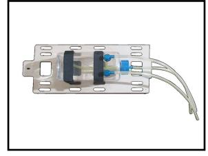
Slide the fuel tank into the fuselage. Guide the lines from the tank through the hole in the fiewall.
