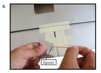
Before the epoxy fully cures, remove the tape from around the control horn. This will allow the epoxy to flow around the control horn, creating a small filet between the control horn and surface for a filshed look and secure bond.
