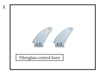
Use sandpaper to scuff the bottom of the aileron and flap control horns. Use a paper towel and isopropyl alcohol to remove any oils or debris from the control horns.
