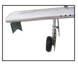
Secure the landing gear doors to the landing gear struts.
