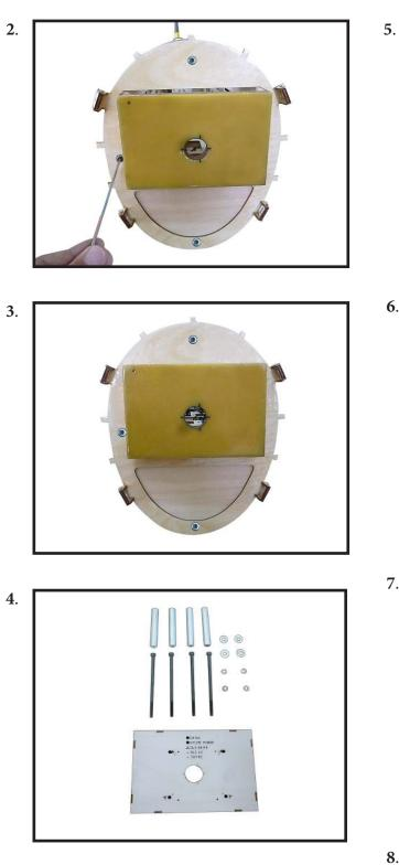
Locate the engine mounting in position on the firewall. Use a 2.5mm drill bit to drill the holes necessary to mount your particular motor choice.
