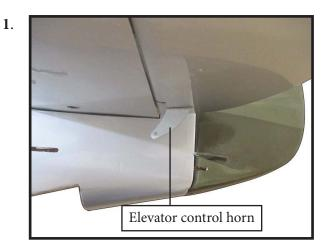
Thread one clevis and M3 lock nut on to each elevator control rod. Thread the horns on until they are flush with the ends of the control rods.
