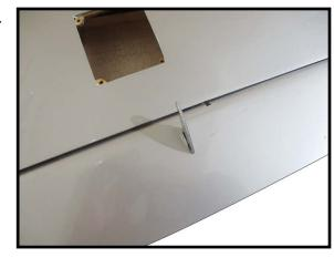
Place low-tack tape 1/32 inch (1mm) from the control horn slot. This will prevent epoxy from getting on the control surface when the control horns are glued in place.
