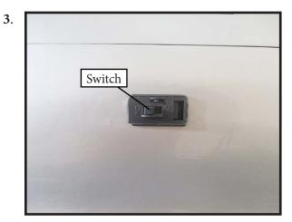
INSTALLING THE ENGINE SWITCH
