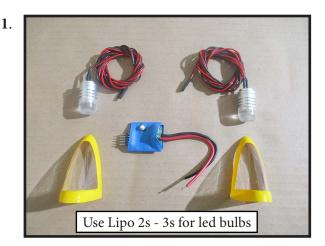
The Blue light for right wing tip, and the red light for left wing tip. They are designed to operate on voltages 7,4v - 12v. Connect lights into switch circuit so that optional the different flashes mode.
