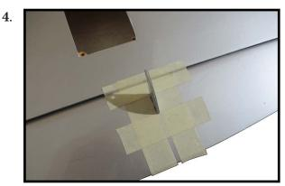
Remove the control horns from the control surfaces. Apply epoxy to the slot in the aileron and flap. Make sure the epoxy gets into the slot for a good bond between the surfaces and control horn.
