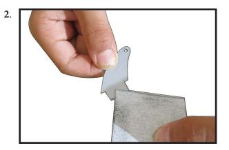
Check the fit of the control horns to the aileron and flap. They should rest flush against the control surface as shown.
