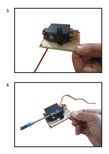
Attach the flap linkage to the control horn. Slide the clevis retainer over the forks of the clevis.
