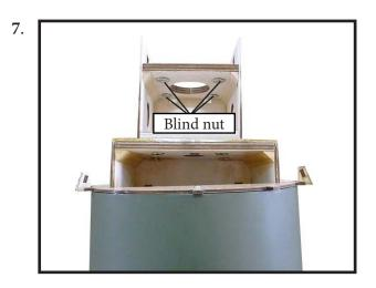
Attach the motor to the front of the electric motor box using four 5mm blind nut, four M5x20mm hex head bolts to secure the motor. Please see picture shown.
