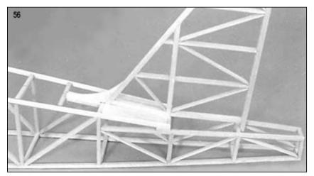
NOTE: The top of FT must be thin for proper tank position. The front FT is supported by the firewall. The rear one by the 3/16" sq. crosspiece behind it. Brace the center FT with scrap hardwood so that it will withstand the pressure of applying the top sheeting.
