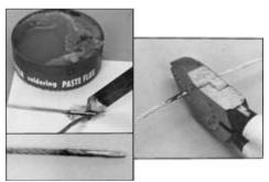
length is arrived at, sweat solder the area to be cut so that it will not fray and unravel while being cut. It can be cut with a good pair of side-cutting pliers, filed in two, ground through on the edge of a grinding tool, or cut with a silicon cutting wheel on a motor tool.
