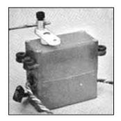
The Sig Pushrod Connector included in this kit can be used for attaching the nosewheel pushrod cable to the steering arm as shown. Additional pushrod connectors can be purchased (Sig No. SH-736) for use on the throttle and nosewheel servo arms. Adjust by loosening the set screw and sliding the cable.
