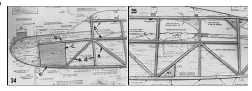
NOTE: The cabin top spruce pieces are precut. Do not cut up longer pieces of spruce for the cabin top. Make certain you understand the location of the spruce pieces in the fuselage before beginning to build it by studying the plan.
