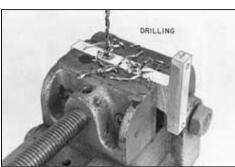
Run the drill at a moderate speed with moderate pressure. Let the bit cut its way through the aluminum at its own rate. Don't try to force it with excess pressure or high speed. Aluminum galls easily and may jam and break the bit if forced. If resistance builds up, back it out of the hole frequently and clean off the metal fragments. Relubricate the bit and hole with oil and continue drilling.
