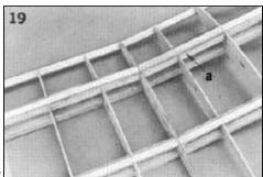
Use slow setting epoxy and work these holes full of glue with a wire. Then coat the faces of the spars. I.e. trailing edge and rib roots, and join the wing halves together. The holes full of epoxy will "nail" the spars together. If the wing ever breaks it will not be on the center line.
