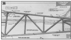
Build the second fuselage side directly on top of the first side, using pieces of wax paper at each point to keep from gluing the sides together. Remove the sides from the board and mark a left and right side so as to insure the next step is done correctly.
