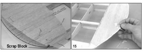
17. Trim the leading edge block off as shown and sand and smooth. This shape is determined by the trimming and rounding of the leading edge. Do not shape the leading edge at the center section until after the windshield fillet is glued on later.
