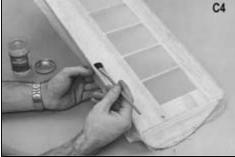
Brush around the outside edge of the stretched silk with clear dope. The dope will soak through the material and adhere to the dope already dried into the framework.
