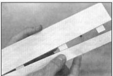
attached but not glued. Align the two surfaces and adjust the gap between them as required. For best control response, the gap should generally be as small as possible but big enough to allow the control surface to move to the maximum deflection that you require.
