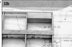
33 a. True up one edge on each of two 1/16"x1-1/2"x24" balsa sheets and cut them down to 1" wide by trimming the second edge. Glue one piece to the bottom trailing edge of each rib. Use the glue sparingly so that you don't glue the partially cut jigging tabs to each rib. Now glue the other piece to the top trailing edge of each rib.
