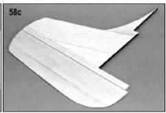
c. Mark a centerline around the tip of the rudder. Using the centerline as a guide taper the trailing edge of the rudder to a constant thickness. Round off all of the edges of the rudder.
