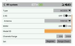
The system will assign you the receiver a number automatically, when you create a new model, and this can be easily changed. The range of the Model ID is 00-63, with the default number being 01. Once the receiver is set to the desired number and is bound to the TANDEM X20S, the bind procedure will not need to be repeated unless the receiver number is changed. At this point, set the receiving number to your preferred number and repeat the binding operation.
