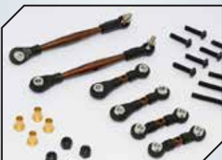
Art.Nr.: GPMWW2160STOCBEBK GPM Federstahl Spurstangen m. Kugelpfannen (6 Stk.) f. Tamiya Wild Willy 2
