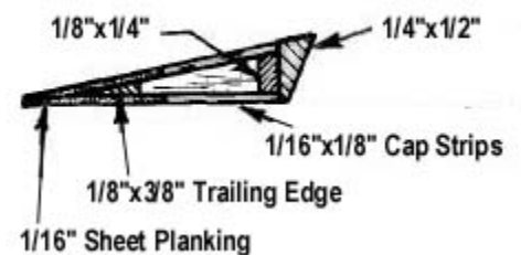
Aileron Rib Cross-Section
