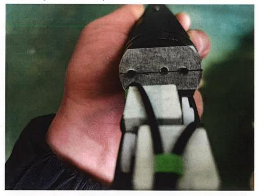
Insert the pull rod guide in the attachment and position it with glue
