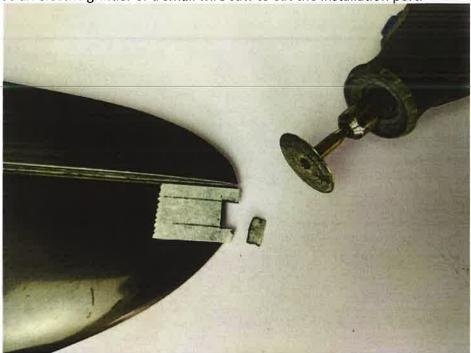
Use tools such as bent steel wire and small file to clean the core in the corresponding area of the wing tip with reference to the auxiliary line, so that there is no residual core foam between the hand buckle inserted into the wing part and the wing carbon structure.
