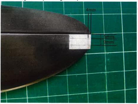
Use an electric grinder or a small wire saw to cut the installation port.
