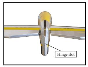
Slide the vertical stabilizer into the slot in the top of the fuselage. The rear edge of the stabilizer should be flush with the rear edge of the fuselage and the lower rudder hinge should engage the precut hinge slot in the lower fuselage. The bottom edge of the stabilizer should also be firmly pushed against the top of the horizontal stabilizer.
