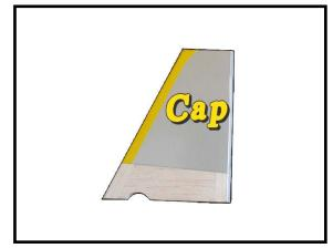
When cutting through the covering to remove it, cut with only enough pressure to only cut through the covering itself. Cutting into the balsa structure may weaken it. Slide the vertical stabilizer back inplace. Using a triangle, check to ensure that the vertical stabilizer is aligned 90° to the horizontal stabilizer.
