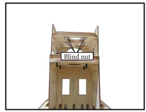
Attach the motor to the front of the electric motor box using four 3mm blind nut, four M3x20mm hex head bolts to secure the motor. Please see picture shown.
