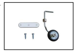
Test fit the tail gear to make sure that it fits properly. When you are happy with the fit, attach the tail gear using the two M3x20mm wood screws.
