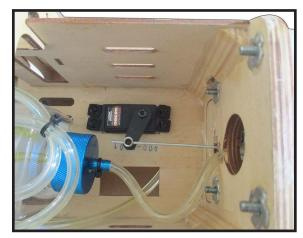
Move the throttle stick to the closed position and move the carburetor to closed. Use a 2.5mm hex wrench to tighten the screw that secures the throttle pushrod wire. Make sure to use threadlock on the screw so it does not vibrate loose.
