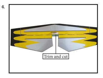
When cutting through the covering to remove it, cut with only enough pressure to only cut through the covering itself. Cutting into the balsa structure may weaken it.
