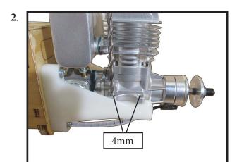
Use a drill to drill the four holes in the engine mount rails.
