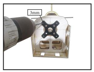
Then, use 3mm drill bit to enlarge the holes on the electric motor box.
