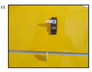
Reinstall the servo into the servo mount and secure the servo inplace using the wood screws provided with you radio system.
