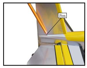
Remove the stabilizer. Using a modeling knife, remove the covering from below the lines you drew.
