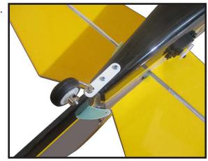
Hold the rudder in place and mark it
