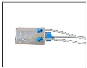
You should mark which tube is the vent and which is the fuel pickup when you attach fuel tubing to the tubes in the stopper. Once the tank is installed inside the fuselage, it may be difficult to determine which is which.
