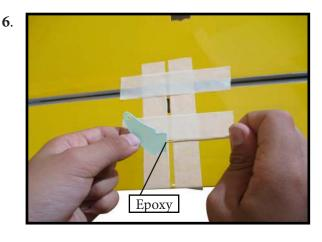
Before the epoxy fully cures, remove the tape from around the control horn. This will allow the epoxy to flow around the control horn, creating a small filet between the control horn and surface for a fiished look and secure bond.
