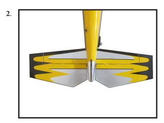
With the stabilizer held firmly in place, use a pen and draw lines onto the stabilizer where it and the fuselage sides meet. Do this on both the right and left sides and top and bottom of the stabilizer.
