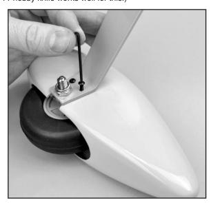
□ 11) Attach the landing gear to the bottom of the fuselage using three M4 x 20mm Socket-Head Bolts and three M4 Flat Washers.
