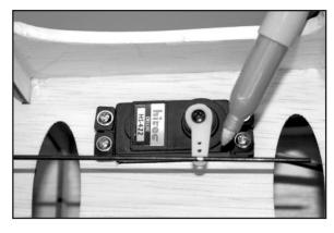
d) Unclip the clevis from the rudder control horn so that you can now pull as much of the wire pushrod forward into the radio compartment as possible, to make is easier to finish the servo end of the pushrod. Mark and cut the servo end of the pushrod wire1/4" past the mark you made in the last step. Then use a pliers to put a 90-degree bend in the wire.
