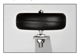
□ 10) Check the orientation of the landing gear to make sure you know which way is forward. The two outer holes for mounting the gear to the fuselage go to the front. Then test fit the wheel pants over the wheels and line up the predrilled mounting holes. Secure the wheel pants in place with two M3 x 10mm socket head bolts for each pant. (You may need to clean a little paint out of the blind nuts inside the wheel pants in order to start the mounting bolts. A #11 hobby knife works well for this.)
