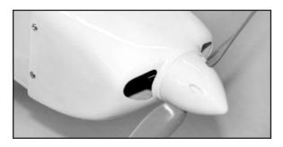
Some of you may decide to leave the plastic spinner off to allow more cooling air to enter the cowling around the prop shaft. If so, be sure to use an "acorn" style prop nut for safety.
