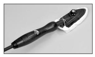
We suggest using a model airplane covering iron for this process. Cover the iron's shoe with a thin cotton cloth, such as an old tshirt, to prevent scratching the covering as you work.
