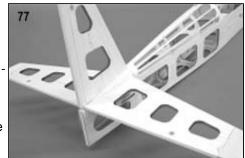
77. Before gluing the left and right fin fairing blocks in place, use a single edge razor blade to carefully notch the fin tailpost to clear the elevator joiner wire. This notch should be cut to the trailing edge of the stablizer and 1/4" width. Once satisfied, glue the fin fairing blocks in place to the fin, stab and back of F-7. Use a small sanding block with 220 grit sandpaper to blend the fairing blocks smoothly to the contours of F-7.
