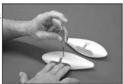
f. Apply glue to the inner face of the mounting plate and glue it inside the wheel pant, with its two mounting holes lined up with the two holes drilled in the pant - use the 4-40 x3/8" bolts to tighten the plate to the inside surface of the pant.
