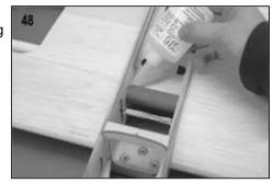
Repeat the procedure to mount the remaining wing panel. Hook a #64 rubber band to one of the J-hooks and stretch the rubber band three times between each hook to seat the wing panels in place. Check the relationship of the wing panel root ribs to the fuselage sides - they should be flush with no gaps. With the wings still attached, apply glue to the inside female wing tube/fuselage side joints. Also apply glue to the female wing tube, where it meets the front edge of the servo tray.
