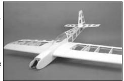
BUILDERS TIP: We suggest that you DO NOT seal the inside of the tank compartment before you cover the fuselage. Applying a sealer of any kind (epoxy resin, etc.) to the inside surface of the wood prevents heat from passing through it and can cause bubbling. Even though it is a bit more difficult, seal the tank area after the fuselage is covered.
