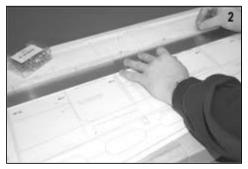
BUILDERS TIP: When pinning ribs to your work surface, pin them in place through each side of the removable alignment/standoff tabs on the bottom rear.
