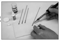
BUILDERS TIP: For a really nice look, use a good metal polish, such as "Simichrome" or "Flitz" to polish these support wires and solder links to a high luster, chrome-like finish.
