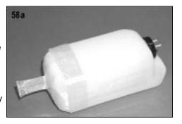
Access to the tank is easy if you use filament strapping tape to create a rear tab that allows you to grasp it and pull the tank out if needed. To do this, use alcohol to first clean the outside of the tank. Then wrap the length of the tank one or two times with strapping tape. Then wrap a third time, folding a 1-1/2" - 2" tab at the rear. The tab gives you a nice grip on the tank in order to easily pull it out.
