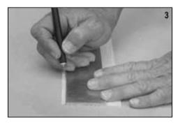
NOTE: Harder sheeting may need to be wetted before bending it into place, to prevent cracking. Warm water sponged onto the outer surface will cause the sheeting to swell, allowing it to conform easily to the rib contour.
