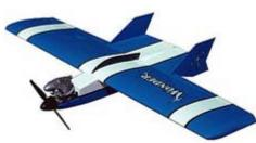
The Standard Wonder is probably the most generic-looking version, but it was the original. All of the other versions were an offshoot of the Standard. Its most distinctive feature has to be the down-turned vortex wingtips. The wingtips probably don't do much aerodynamically for a model of this size, but they do look good and generate lots of comments from fellow modelers.
