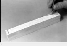
3. Carve and sand the wingtip blocks to match the contour of the entire upper surface and back to the spar on the lower surface.
