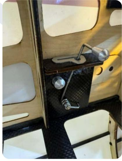
To lock the elevator in place just move the EZ-Quick release pin forward, slide the elevator in place and release the pin. make sure you give the elevator a tug to make sure the system is in the locked position.
