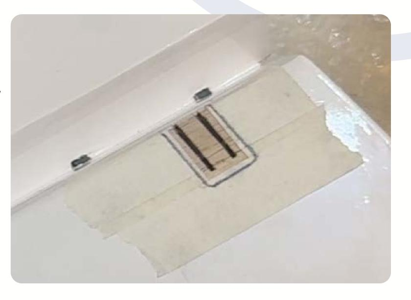
Apply 30 minute epoxy to the slots and thoroughly coat the horns and base plate bottom. Reinsert the assembly into the slots and wipe away any excess epoxy with a paper towel and alcohol. Place a 3mm bolt through the horns to help ensure proper alignment and set aside to dry.
