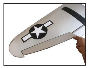
Check the fit of the aileron to the wing. The top of the ailerons will align to the top of the wing. Make sure movement is smooth and bind free.
