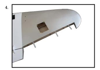
Insert all four hinges in the ailerons at this time. Make sure hinges move up and down in right direction and not side to side!
