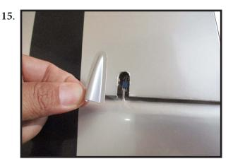
Use canopy glue to attach the cover to the wing. Use low-tack tape to keep the cover in position until the adhesive fully cures.
