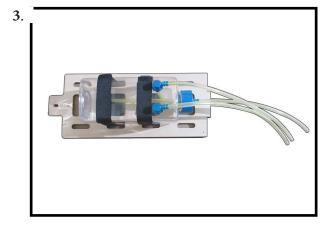
Slide the fuel tank into the fuselage. Guide the lines from the tank through the hole in the fiewall.
