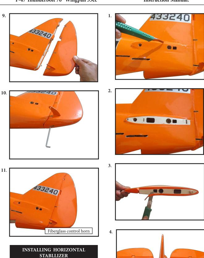
Use Epoxy Glue to glue the Horizontal Stabilizer to the fuselage.
