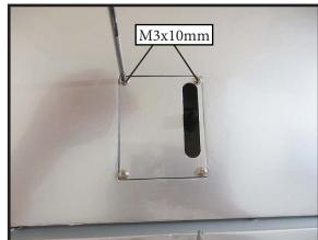
Set the aileron hatch in place and use a
