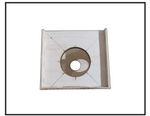
Attach the motor mount to the front of the electric motor box using four 5mm blind nut, four M5x30mm hex head bolts to secure the motor. Please see picture shown.
