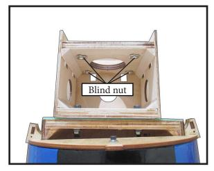
Attach the motor to the front of the electric motor box using four 5mm blind nut, four M4x20mm hex head bolts to secure the motor. Please see picture shown.
