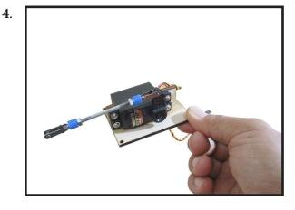
Attach the flap linkage to the control horn. Slide the clevis retainer over the forks of the clevis.
