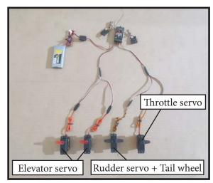
Secure the servos with the screws provided with your radio system.
