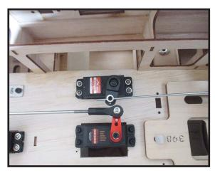
Reinstall the servo horn by sliding the connector over the pushrod wire. Center the throttle stick and trim and install the servo horn perpendicular to the servo center line.
