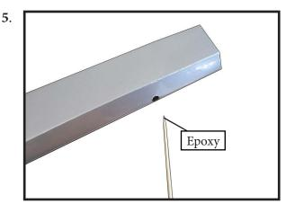
Apply epoxy into each of the holes in the ailerons using a spare piece of pushrod wire or toothpick.
