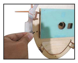
Connect the lines from the tank to the engine and muffler. The vent line will connect to the muffler and the line from the clunk tothe carburetor.
