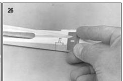
27. Die-cut 3/32" plywood servo rails (SR-1, SR-2, and SR-3) have been provided. Trim the servo rails if necessary to fit your particular servos. Epoxy the rails in place in the fuselage between formers F-2 and F-3. Mount the servos to the rails in the manner recommended by the radio manufacturer.
