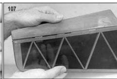
107. At this point the stabilizer and elevator are joined on the EASY HINGES, but the hinges are not glued. Align the stab and elevator, then adjust the gap between them as required. For best control response, the gap should generally be as small as possible but big enough to allow the control surface to move to the maximum deflection that you will require.
