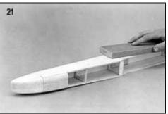
22. The fuselage is now ready for final sanding. Sand off all "Tee-Lock" stubsa and round the edges of the fuselage with a sanding block. Start out with 150 grit sandpaper and switch to 220 grit sandpaper for the final sanding.
