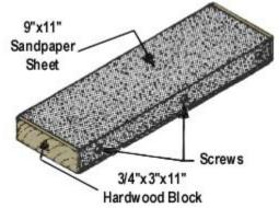
Finally, glue sandpaper onto different sizes of scrap plywood sticks and round hardwood dowels. These are handy for working in tight places and for careful shaping where a big block is too hard to control.
