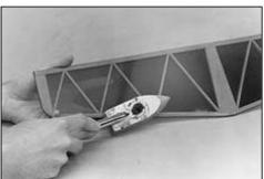
104. Cover the bottom side of the elevators first and then the top. When covering solid sheet surfaces like the elevators, better results may be obtained by starting at the center and working toward the outer edges. This allows the air to escape from under the covering as it is applied.
