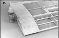
NOTE: If you want to use the "Optional Bolt-On Wing Attachment" method described in the next step, do not glue the foremost top and bottom pieces of 1/16" sheeting that contact the leading edge in place at this time.
