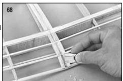
69. Regardless of whether you have elected to use the optional bolt-on wing attachment or the standard rubber band wing mounting, glue the die-cut 1/16" plywood trailing edge reinforcement (TR) piece in place on top of the trailing edge at this time.
