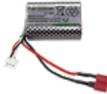
7.4V 1,500mAh rechargeable battery
