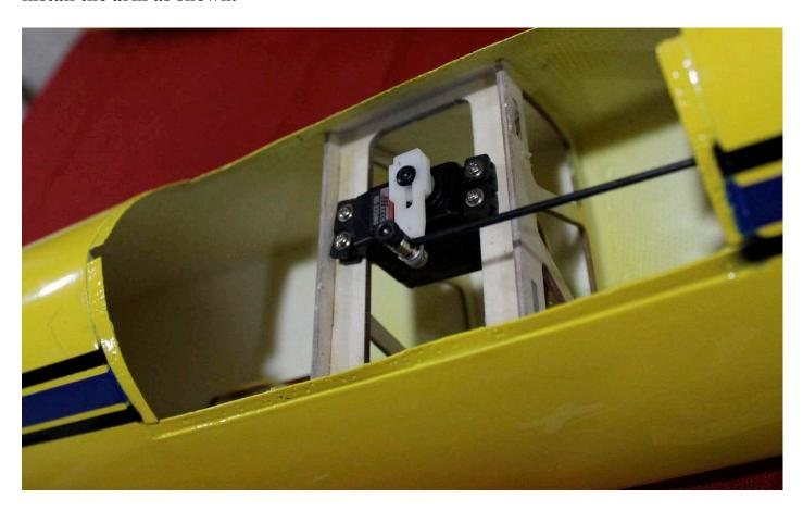
13. Locate the front mount on the float with the servo installed and modify the slot as shown by lengthening it a few mm as shown to allow the servo extension to exit.
