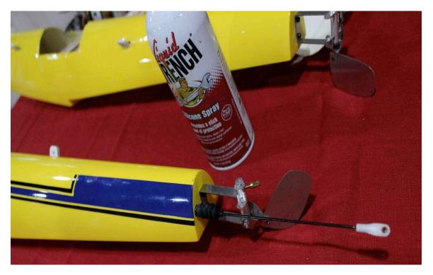
9. Using a 2mm screw and nut, with Loctite, attach the ball link to the water rudder arm as shown.
