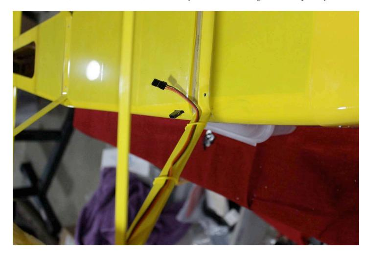
23. It is wise to package your receiver and ESC inside plastic bags, using caulk to seal the wire exists, before float-flying.
