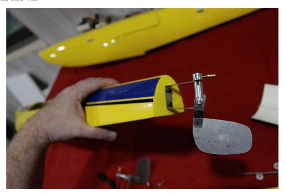
5. Locate the left float – The strut mounts extend to the inside, the left float has its mounts on the right side. Place some painter's tape on the rear of the float as shown to minimize paint chipping while drilling for the pushrod exit.
