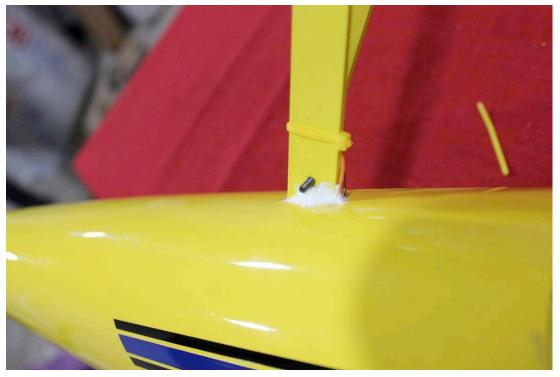
18. Attach the cross-rod between the water rudders as shown, making sure rudders are in perfect alignment.
