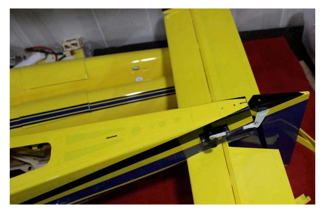
3. If you are permanently converting to floats, glue the sub-fin into the fuselage as shown. If you intend to switch back, we recommend using Blenderm tape to secure the sub-fin to the fuselage, one strip one each side along the joint.
