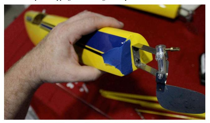
6. Drill a pushrod exit hole as shown to align with the water rudder steering arm, starting with a 1/8" (3mm) bit and finishing with a 1/4" (6mm) bit.
