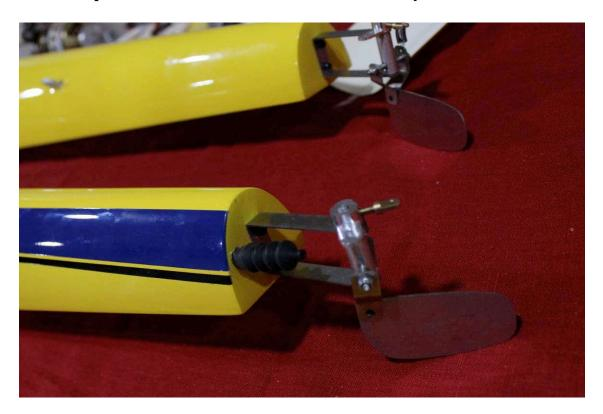
8. Assemble the pushrod by screwing the ball link onto the threaded end as shown. Coat the pushrod in silicone lubricant or oil and push through the bellows seal as shown
