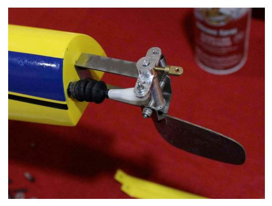
10. Using Loctite on the nut, attach the cross-rod EZ-connector to the water rudder as shown, loose enough that the connector can easily spin. Do this on both floats.
