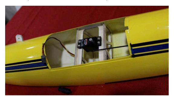
12. Install a pushrod EZ-connector onto your servo arm, loose enough that it can rotate, using Loctite on the nut to retain it. Electronically center your servo and install the arm as shown.
