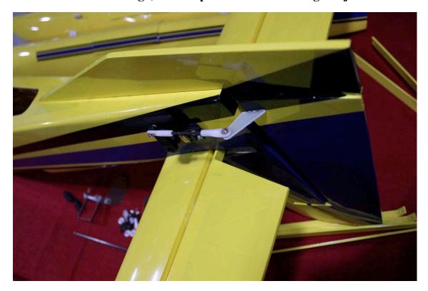
4. Install the water rudders onto the rear of the floats using 3mm screws with Loctite as shown.
