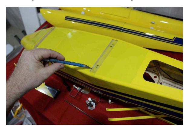
2. Remove the covering over the two slots at the rear of the fuselage as shown.
