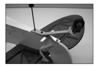
Attach the steering springs to the three armed steering horn and the tailwheel horn.
