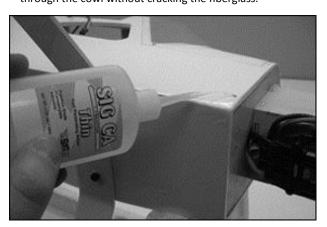
f) The cowl can now be permanently mounted to the fuselage.
