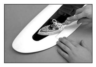
If wrinkles keep coming back on the tail surfaces, you may need to "ventilate" the areas between the ribs. Otherwise the air that is sealed in those relatively small areas will expand when the heat is applied and actually cause the covering to stretch instead of shrink. Use a pin to poke a tiny hole in the covering between each rib, on the bottom of the part. That will let the expanding air escape and the covering to shrink properly.
