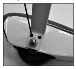
☐ 10) Attach the landing gear to the bottom of the fuselage using three M4 x 20mm Socket-Head Bolts and three M4 Split-Ring Lock Washers.
