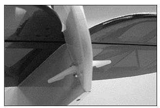
□ 18) There are three holes pre-drilled in the <u>RIGHT</u> side elevator for mounting a nylon control horn. Screw the control horn in position on the bottom of the elevator, with the retaining plate on the top, using three M2 x 14mm Screws and three M2 nuts, making sure to add a drop of thread locker to each screw before tightening the nut.
