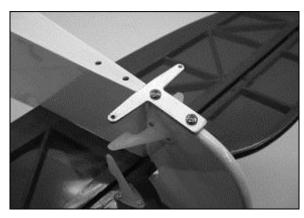
d) Attach the pre-assembled tailwheel bracket to the fuselage using two M3x18mm machine screws and split-ring lock washers. Add a drop of thread locker to each of the M3x16mm machine screws before tightening them.
