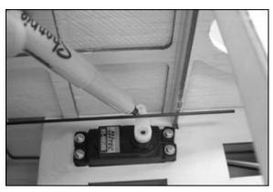
d) Unclip the clevis from the elevator control horn so that you can now pull as much of the wire pushrod forward into the radio compartment as possible, to make it easier to finish the servo end of the pushrod. Mark and cut the servo end of the pushrod wire 1/4" past the mark you made in the last step. Then use a pliers to put a 90-degree bend in the wire at the mark.
