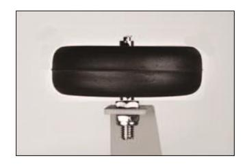
□ 9) Check the orientation of the landing gear to make sure you know which way is forward. The two outer holes for mounting the gear to the fuselage go to the front. Then test fit the wheel pants over the wheels and line up the predrilled mounting holes. Secure the wheel pants in place with two M3 x 12mm socket head bolts for each pant. (You may need to clean a little paint out of the blind nuts inside the wheel pants in order to start the mounting bolts. A #11 hobby knife works well for this.)
