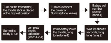
. If R/C throttle signal is reversed, the ESC may enter the calibration incorrectly Please pay special attention to this, power off, reverse the throttle signal and try again.
