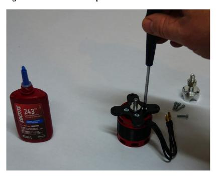
22. Secure the prop adapter using the 4 socket head cap bolts. Again, blue Loctite should be applied to each bolt.
