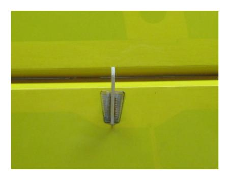
5. Make sure the hinges are centered in their slots. Slide the aileron into position making sure the outer tip of the aileron is flush with the wing tip. Apply a drop of CA at each hinge location on both the top and bottom side of the wing. Use a fresh bottle of thin CA and a fine glue tip for best results.
