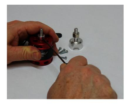
21. Next secure the radial mount to the motor using the provided short Phillip's head machine screws. Again be sure to use a drop of blue Loctite on each screw.
