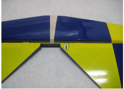
13. Slide the elevator onto the hinges in the stabilizer and secure with thin CA. Again a fresh bottle of CA and a fine glue tip work best here
