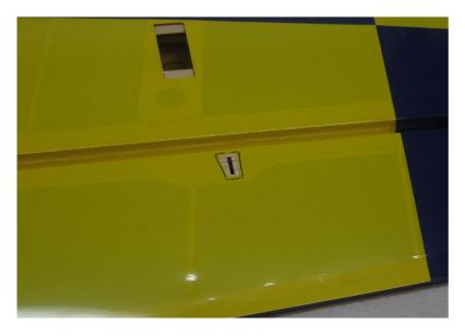
4. Mix up a batch of 30 minute epoxy and apply liberally to the slot in the aileron and to the scuffed portion of the control horn that will insert into the aileron. Install the aileron horn and base plate onto the aileron and wipe away any excess epoxy with a paper towel soaked in denatured alcohol.
