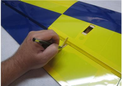
2. Remove the control horn and scuff the portion that will be glued into the aileron with sandpaper.
